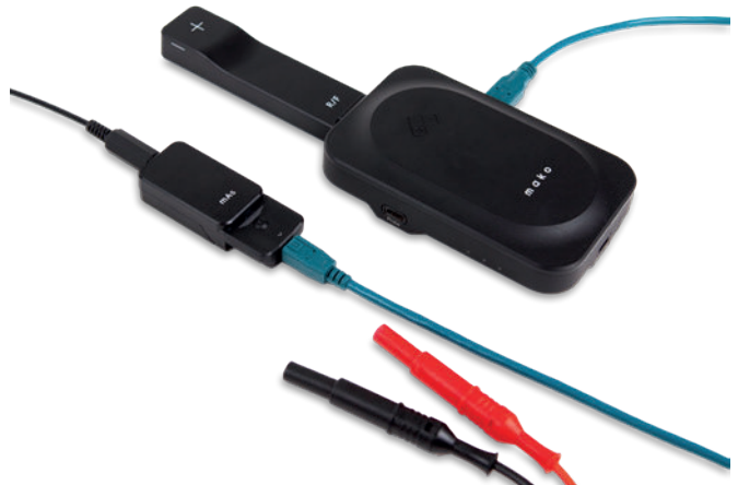
Mako Base Unit with R/F Probe docked, mAs Module connected and mAs cable.
