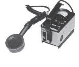
providing instant indication of the radiation level. The Inspector includes an adjustable timer and external calibration controls.
